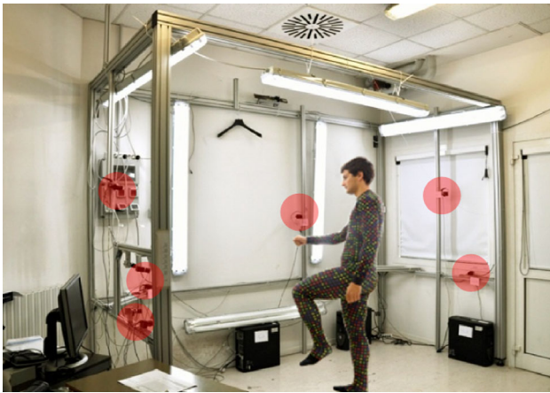
Fig. 1 A picture of the experimental setup together with a test subject wearing the colour-coded garment. Lamps and cameras (circled in red) are attached over the aluminium cage structure. Cameras are linked to the PCs that grab and process the video. The subject is standing in the middle of capture area and he can move freely inside the cage (colour figure online)
